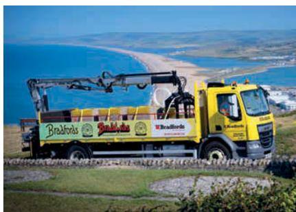
Since 2010, all new lorry loader cranes had to have vehicle stability incorporated into the function of the loader's rated capacity limiter (RCL). RCLs warn (usually acoustically and visually) of an approach to overload at 90% of rated capacity, with a further (different) warning at 100%. The RCL system should either lock out or reduce the lifting capacity in areas where stabilisers have not been fully deployed or there is reduced stability.
